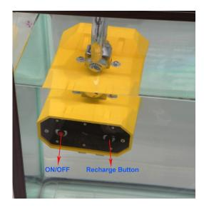
Water proof crane scale OCS-SL is re-equip model based on ordinary crane scale OCS-SL.We take out the two keys(ON/OFF, TARE) of the front panel, and put the ON/OFF key on the back panel. On the back panel, the black button is used for recharging battery. The TARE function can be achieved through the TARE key on the remote control. All other function is just as same as ordinary model, please refer our user manual OCS-SL
